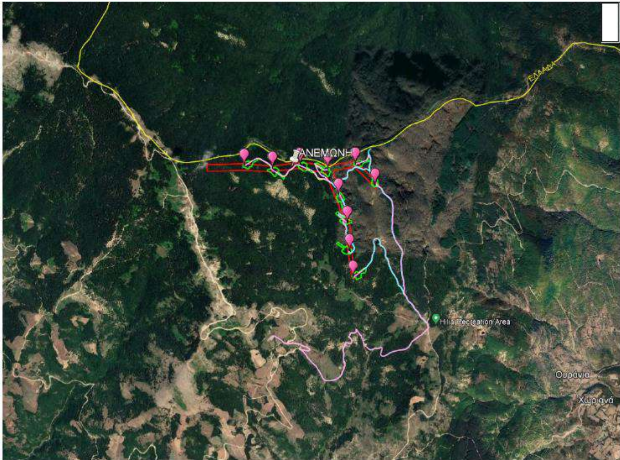
Map 109: Production license polygon of the project under study (red outline), wind turbine installation site (pins in pink), accompanying works (wind turbine squares in green - improvement of existing road network in light blue - new internal openings in yellow) and underground interconnection line in pink which follows the existing road network.
